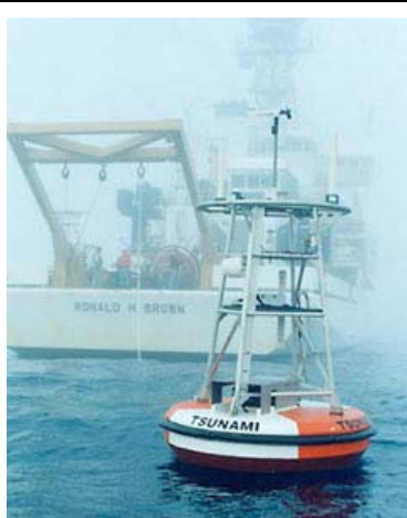
Figure 4.34 A buoy used by the Deep-ocean Assessment and Reporting of Tsunamis (DART) system
