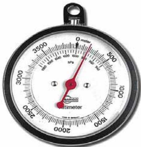
Fig 33: An altimeter Downloaded from http://geometrytech3.wikispaces.com/file on 23/5/11
