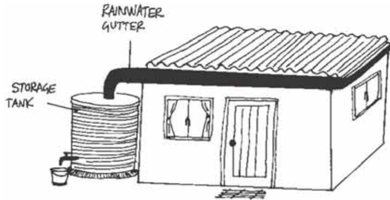
Fig 5: Roof catchment system
