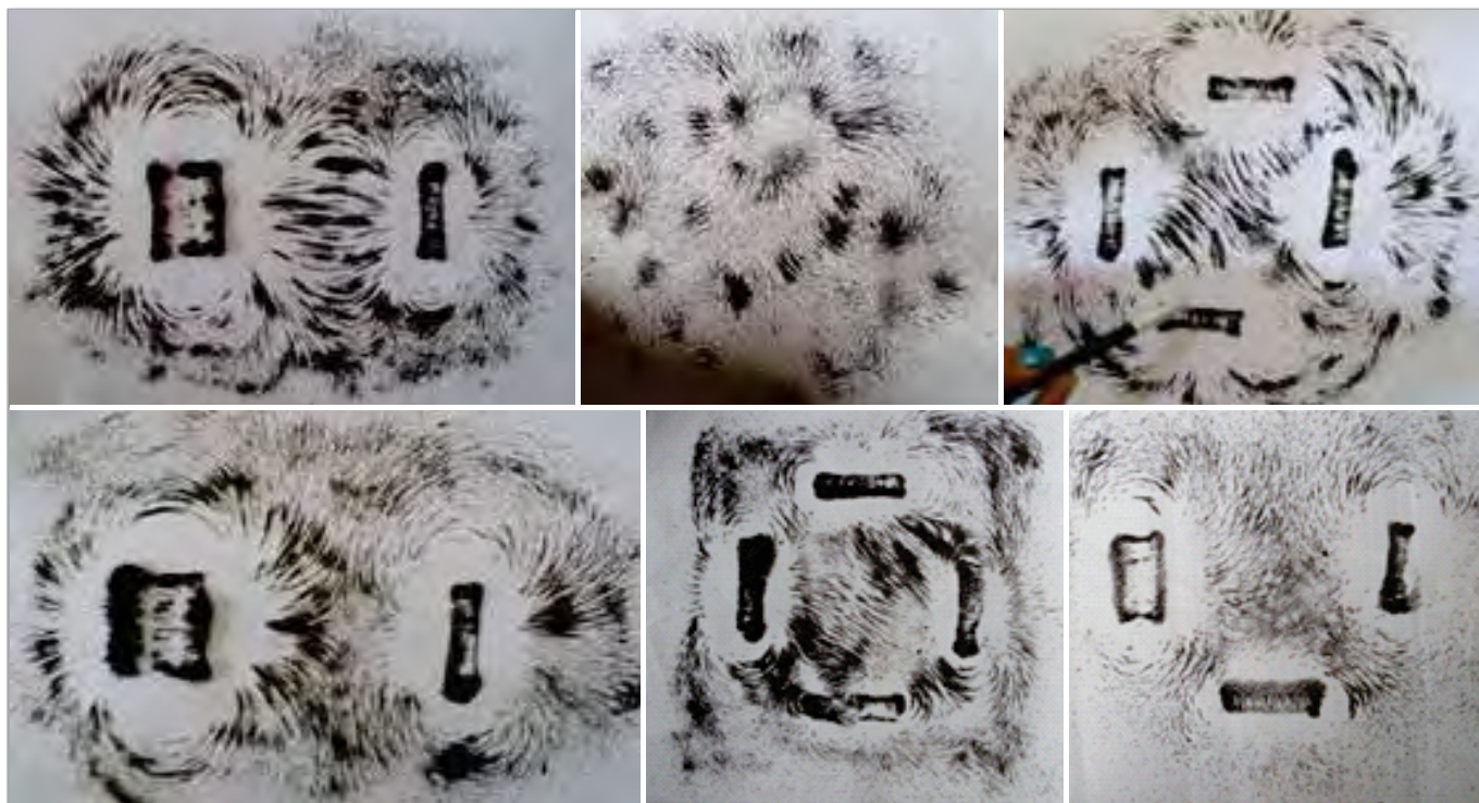
Figure 1. Some pictures of magnetic field lines using iron filings and magnets placed under a sheet of paper. Can you spot opposite poles facing each other above?
